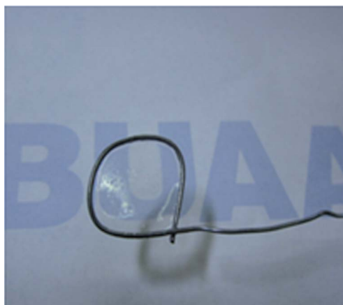
Fig. 4 Digital photograph of free-standing film detached from silicon wafer by dissolving the CA sacrificial layer.
